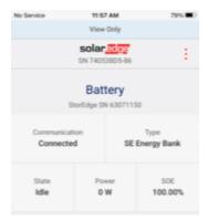
SOC means State of Charge. The state of charge is between 0% and 100% If you overload the battery with instantaneous draw and need to power cycle the system follow the "Energy Hub with Batteries Powercycle process" document
