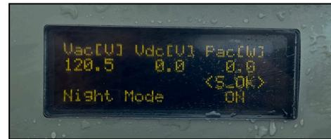
Your inverter should not remain in “Night Mode” during conditions of normal operation.
